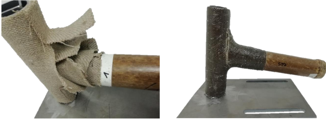
Figure 1 (Left) not yet epoxy impregnated layers of flax fabric around the vertical steel pipe and the bamboo tube of the T-connection. (Right) fractured specimen on the holder after the bending test
