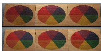
Figure 1 Test pieces: above - without treatment; below – 100 °C, 5% moisture
