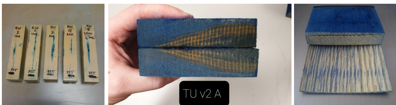
Figure 1 (a) Blue ink distribution in samples of redwood incised into tangential and radial faces, (b) enhanced uptake in heartwood of tulipwood, (c) Southern Yellow Pine plank segment cut to reveal distribution 3mm below the surface
